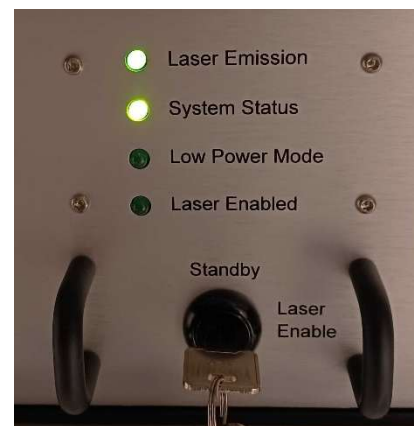
Controller front panel after incorrect power up. Note key position.
