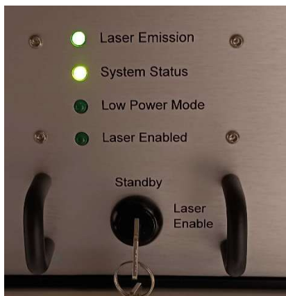
Controller front panel in normal standby mode.
