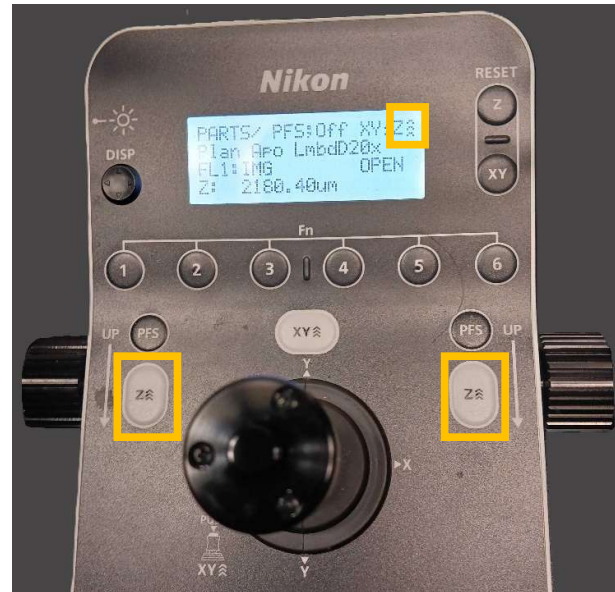
Fig. 2 – Focus Speed Buttons, Coarse Focus Enabled
