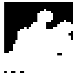
Fig. 17-3 Dilation with kernel size = 7
