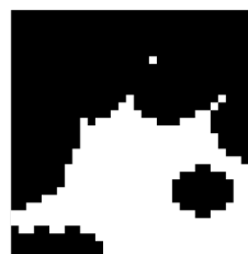
Fig.17-5 Closing with kernel size = 7
